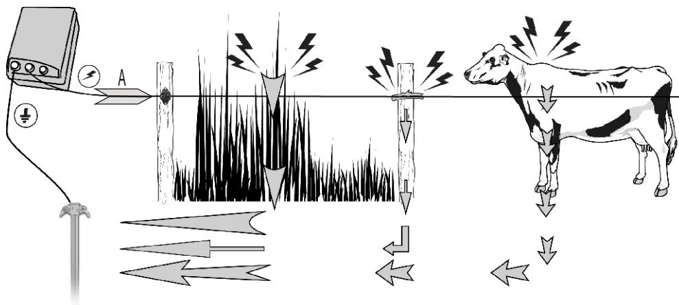
The current leaves the energizer, and circulates through the conductor looking for any way possible to return to earth. The return to the earth can be done via the grass, faulty insulator, animal touching the fence, etc ...
