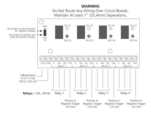
The RL-4 Quad Relay Module provides four independent Form "C" relay contacts. The relays are energized by applying a positive or negative voltage at the input terminal(s). You can choose positive or negative voltage by the setting of the jumper.
